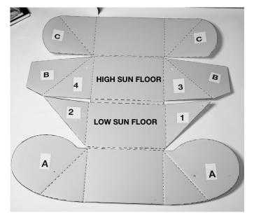
**Step 1** Lay out your cooker shiny side up. Use this image to identify the panels and reflectors. Before you begin assembly, make sure that you have folded all the panels thoroughly. Panels A, C, 1, 2, 3, 4 all fold inward. Panels B fold outward. The more time you spend on this step, the better the end result.
