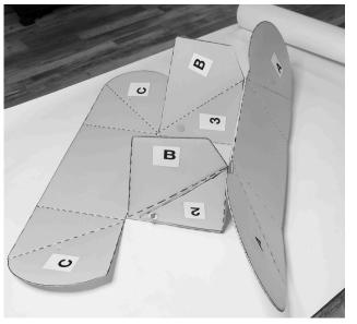
**Step 6** Check your work. Your progress so far should look like the photo above. This is a good time to Fold the B panels outward again. The material is very durable. You will not harm it by flexing
