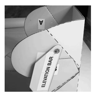
**Step 9** Place an elevation bar on the elevator bolt and hex nut on panel A. Add a steel washer and wing nut. This will secure the elevation bar.
