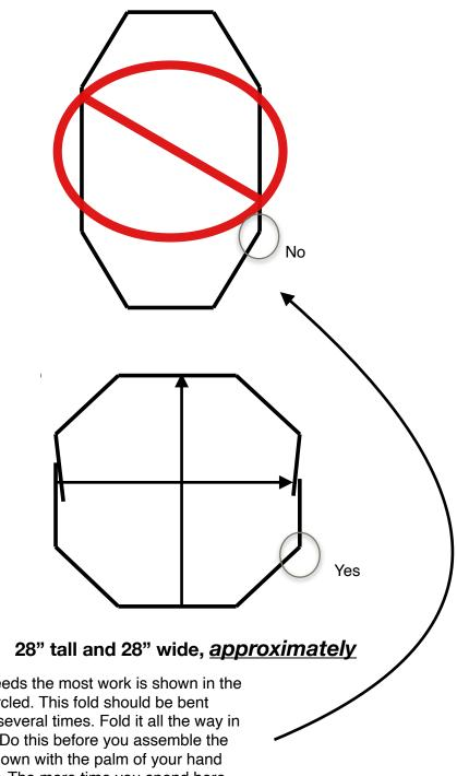
The fold that needs the most work is shown in the top diagram, circled. This fold should be bent back and forth several times. Fold it all the way in each direction. Do this before you assemble the cooker. Press down with the palm of your hand against the fold. The more time you spend here, the better your initial results will be.
