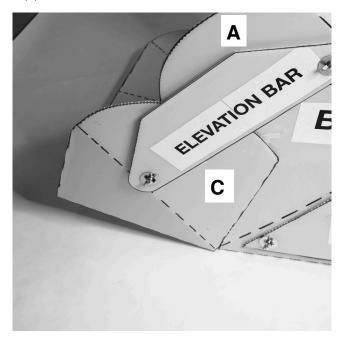
**Step 12** Attach the elevation bar and secure with a steel washer and wing nut. Do not over tighten. This combination of rubber washer, steel washer and wing nut will serve as the "brake" to hold the adjustment position of the cooker. Release the wing nut to make adjustments, tighten the wing nut to hold position. Now, attach the elevation bar for the opposite side of the cooker, keeping in mind the A,B,C assembly order of **Step 10**.
