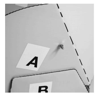
**Step 8** Insert an elevator bolt from the inside of the cooker to the outside. Attach a hex nut as shown
