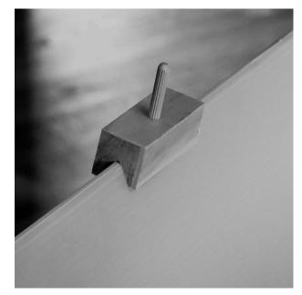
**Step 13** The sunsight is attached to either the bottom reflector or the top reflector. Either one is fine. The fit will be tight, so work the reflector into the sunsight slot by gently rocking the sunsight side to side until the slot is completely filled, as shown.
